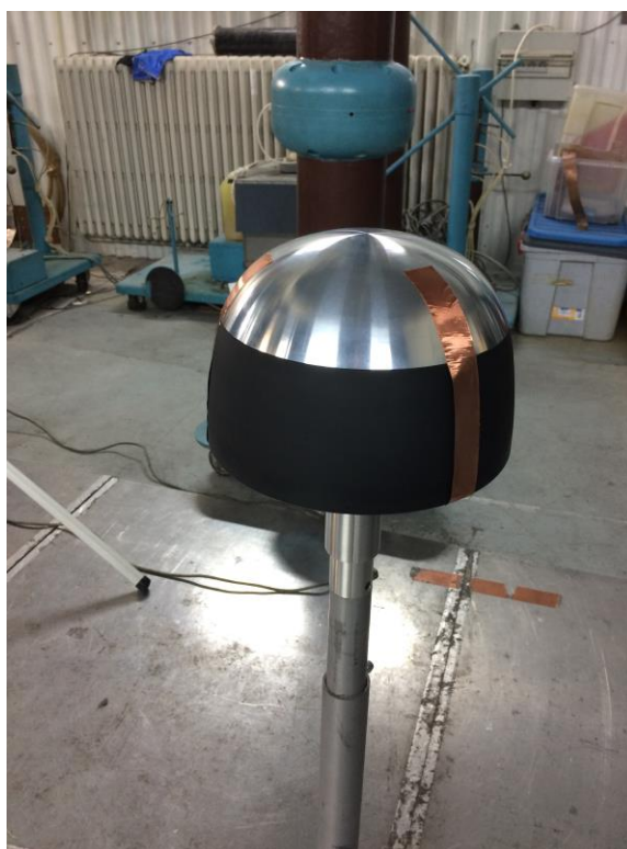
Inactivated DDCE-100-PLUS (short-circuit)
